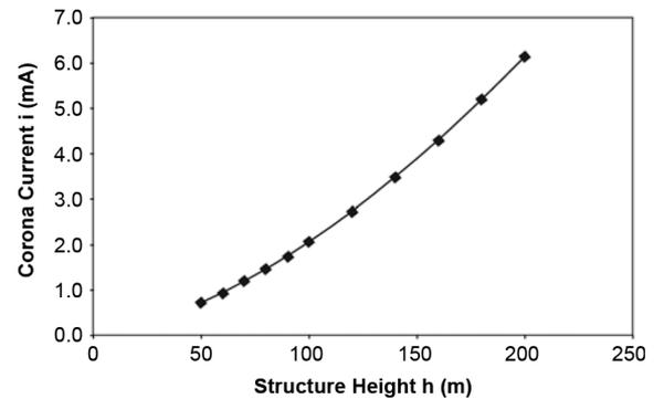
Fig. 9. Corona current variation with structure height,  $a = 1$  m,  $E_g = 20$  kV/m.
