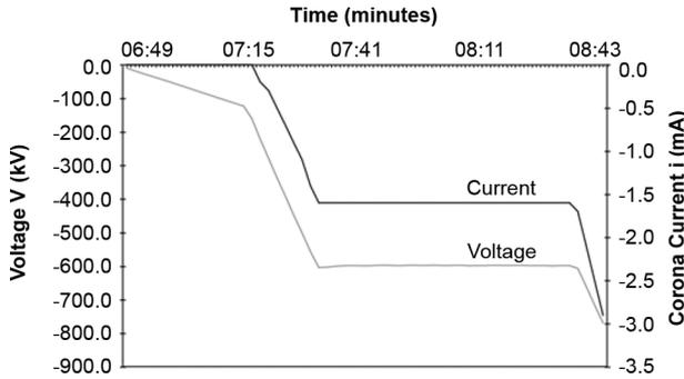
Fig. 5. Measured voltage current characteristics of the wet electrode.
