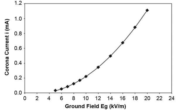
Fig. 7. Corona current from ultra-corona device on 70 m structure  $h/a = 50$ .
