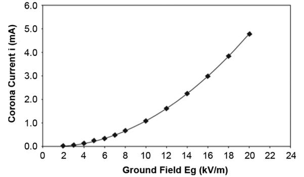
Fig. 8. Corona current from ultra-corona device on 200 m structure,  $h/a = 100$ .
