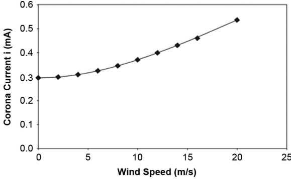
Fig. 10. Effect of wind speed on corona current,  $h = 200$  m,  $h/a = 200$ ,  $E_g = 5$  kV/m.
