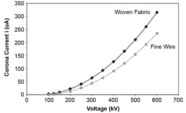
Fig. 6. Corona current-voltage characteristics of double toroids in 3 m gap.
