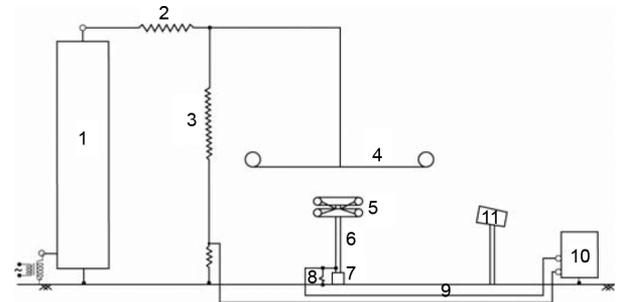
Fig. 3. Schematic diagram of the test circuit and test object. 1: HV cascade rectifier, 2: damping resistor, 3: direct voltage divider, 4: plane electrode, 5: double toroid test object, 6: steel pole, 7: insulator, 8: coaxial shunt, 9: coaxial measuring cables, 10: voltage and current measuring system, and 11: UV camera, video camera, acoustic microphone.
