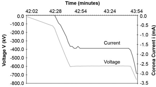
Fig. 4. Measured current voltage characteristics of the dry electrode.
