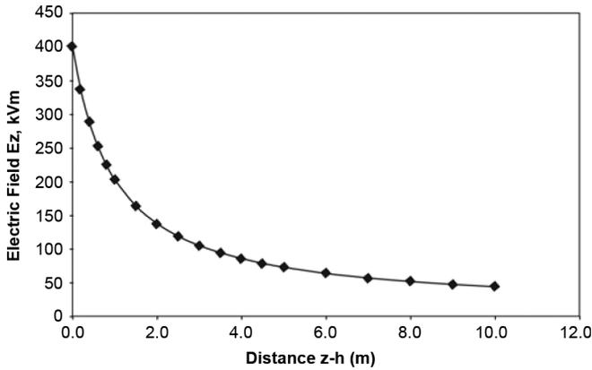
Fig. 2. Variation of axial electric field above structure top,  $h = 150$  m,  $h/a = 75$ ,  $E_g = 10$  kV/m.
