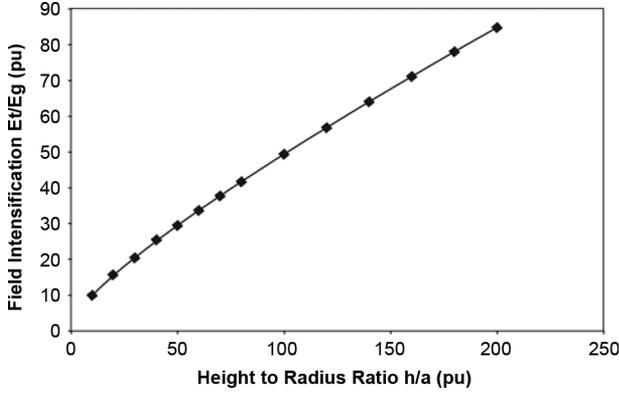
Fig. 1. Field intensification at semi-ellipsoid structure top.
