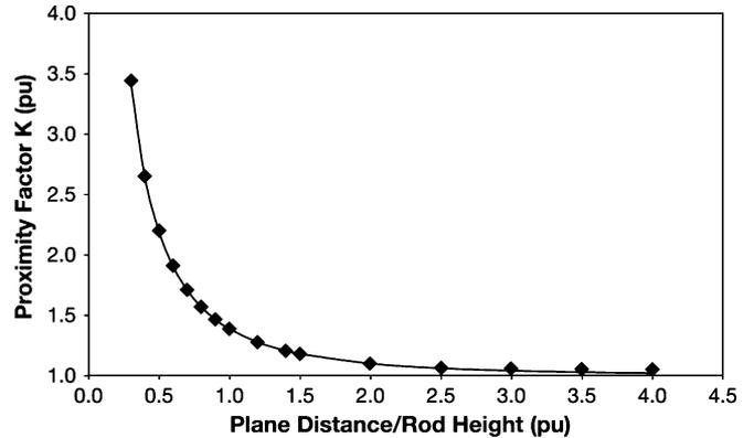
Fig. 9. Variation of parallel plane proximity factor with the plane distance to rod height ratio.
