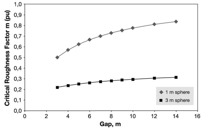
Fig. 7. Effect of sphere-plane gap on the critical surface roughness factor.
