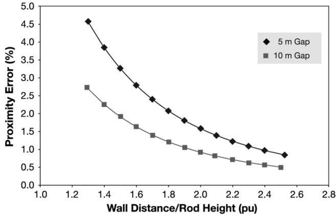
Fig. 3. Dependence of wall proximity error in U50 on wall distance to the rod height ratio under critical switching impulse.
