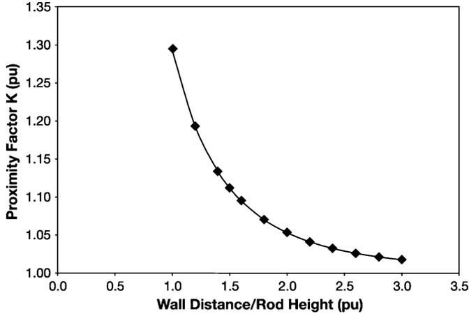
Fig. 2. Variation of wall proximity factor K with wall distance to rod height ratio.
