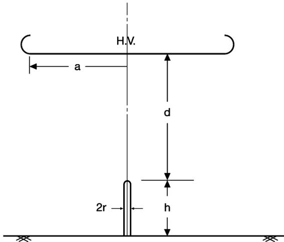
Fig. 8. Schematic diagram of test configuration to determine the critical ground field for continuous leader inception from a vertical rod on the ground plane.
