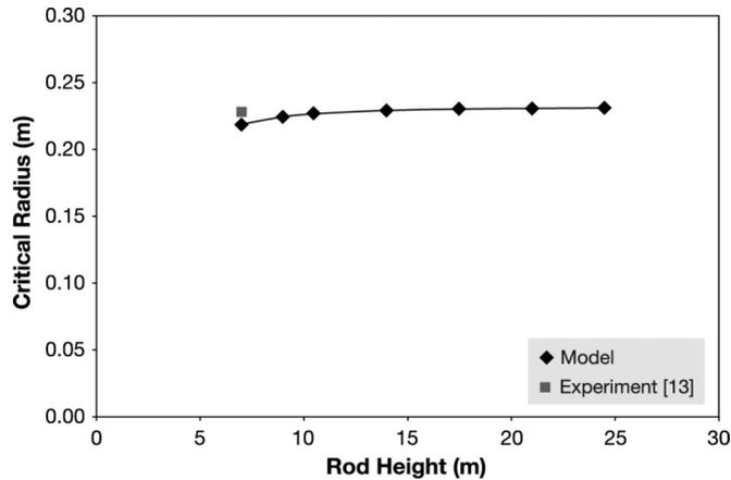
Fig. 11. Variation of critical sphere radius with rod height for 3.5-m rod-upper plane gap.
