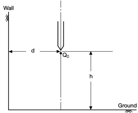
Fig. 1. Rod-plane gap with wall proximity.
