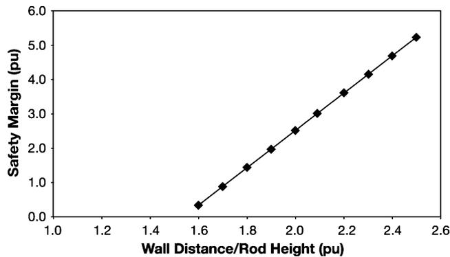
Fig. 4. Dependence of safety margin, in per unit of standard deviation, on wall distance to rod height ratio. 10-m rod-plane gap.
