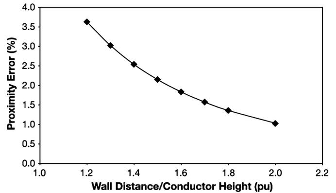
Fig. 5. Variation of the wall proximity error in U50 with the wall distance to conductor height ratio. 10-m conductor-plane gap.
