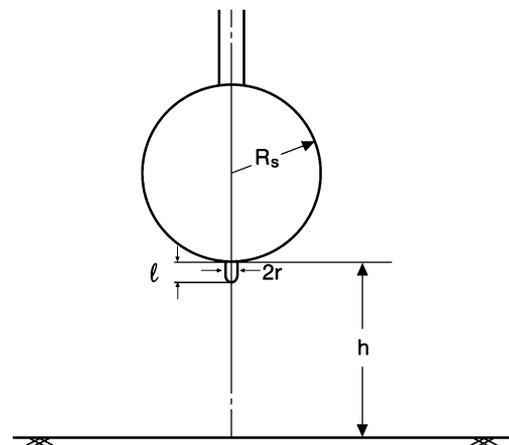
Fig. 6. Simulated protusion in a large sphere-plane gap.
