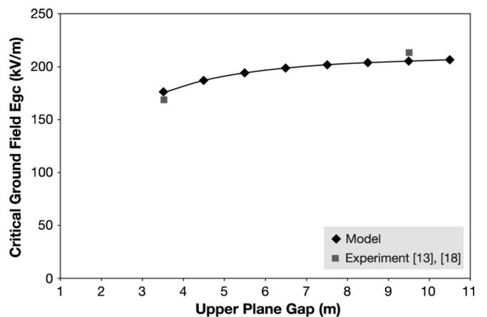
Fig. 10. Dependence of the critical ground field on the rod-upper plane gap. Rod height: 3.5 m.
